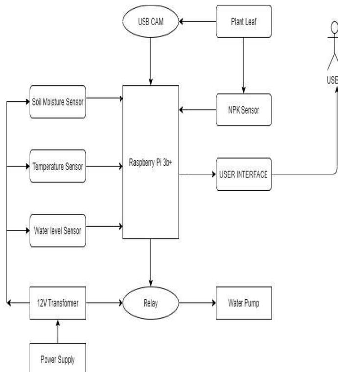
**Figure 1: Block Diagram of Working Model.**
